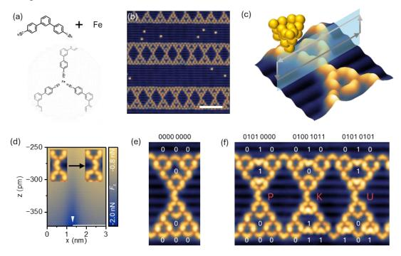
**Figure 1.** (a) Schematic of coordination structure formed by C3PC and Fe atoms. (b) STM iamge of 1D fractal Sierpiński triangle chains. (c) Schematic of tip manipulation to switch the adsorption site of C3PC. (d) Force line spectrum during the tip manipulation. (e) Definition of information sites in a 1D fractal Sierpiński triangle chain. (f) Binary encoding of PKU demonstrated in the 1D fractal Sierpiński triangle chain.
